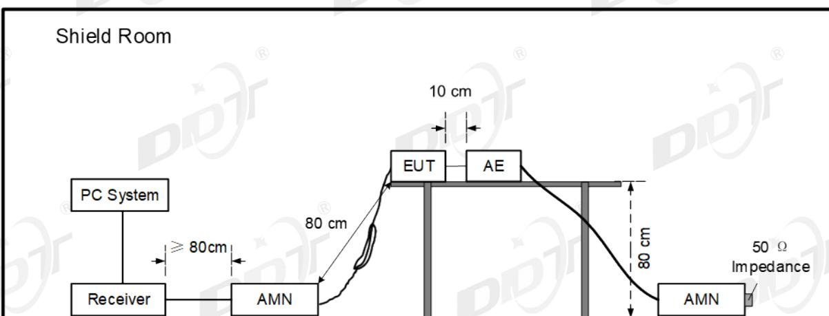
The EUT was placed on a non-metallic table, 80cm above the ground plane. The EUT's power adapter was connected to the power mains through a line impedance stabilization network (AMN). which this provided a 50-ohm coupling impedance for the EUT (Please refer to the block diagram of the test setup and photographs). Both sides of power line
